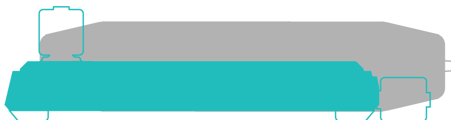
Figure 1. Each Vivaflow® SU cassette (teal) uses 30.5% less plastic than the previous generation Vivaflow® 50 (grey).
