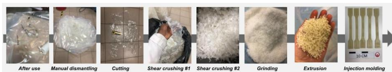
Figure 3. Steps of material preparation of rLDPE_Pure.
