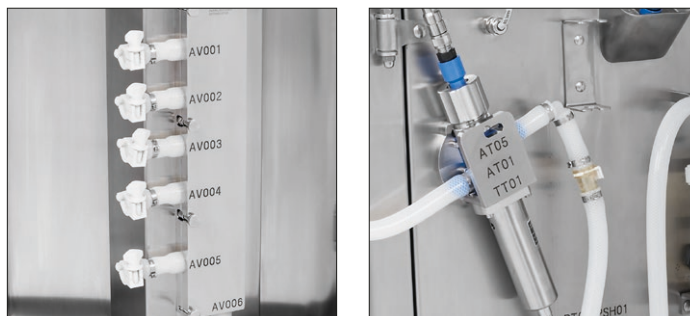
Figure 4: Pinch Valve Buffer Inlet Block (Left); Compact Single-Use Flow Cell (Right)
