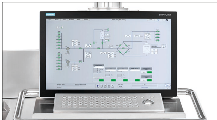
Figure 3: Fully Maneuverable Touchscreen Human Machine Interface (HMI)
