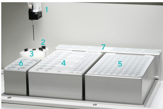
**Figure 3-7:** Sample Chamber Components
