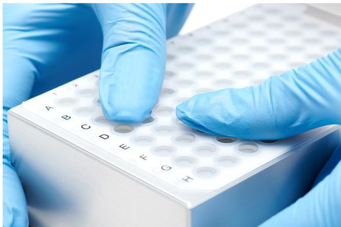
Figure 12-3: How to Grip the Sample Rack
