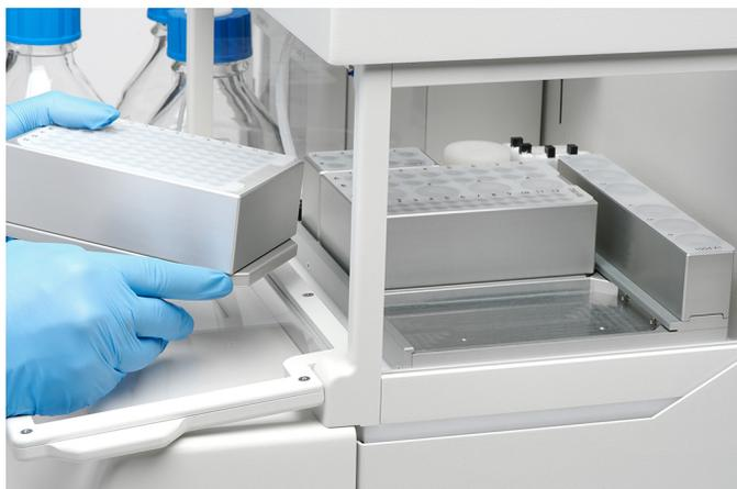
**Figure 3-9:** Installation of Sample Rack
