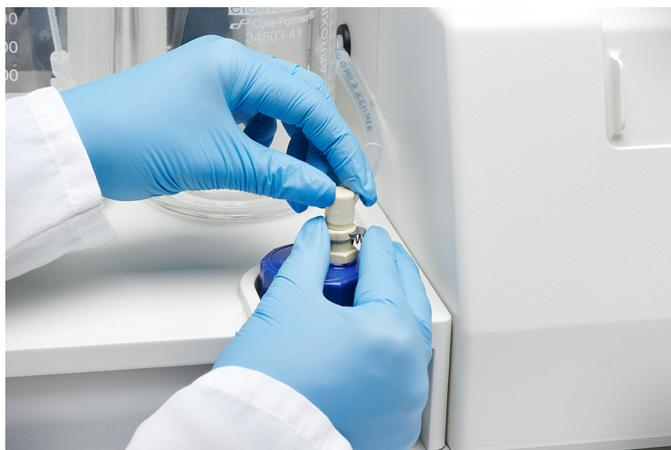
**Figure 12-5:** Removing Waste Tube Connector
