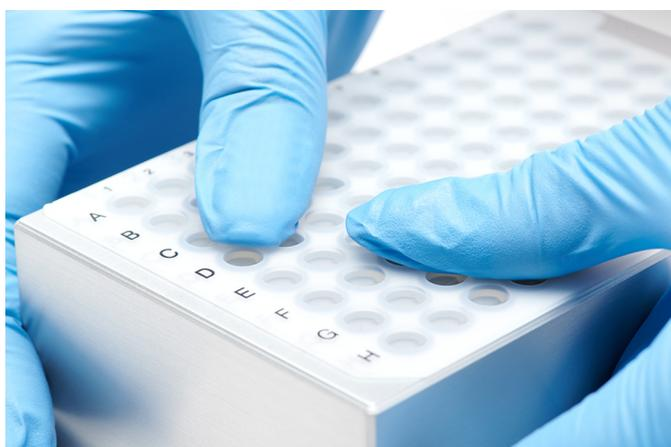
**Figure 3-10:** Installing Septa
