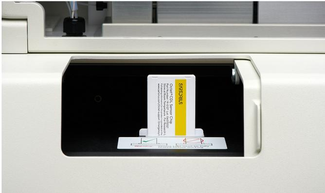
Figure 3-4: Sensor Chip Installation Port
