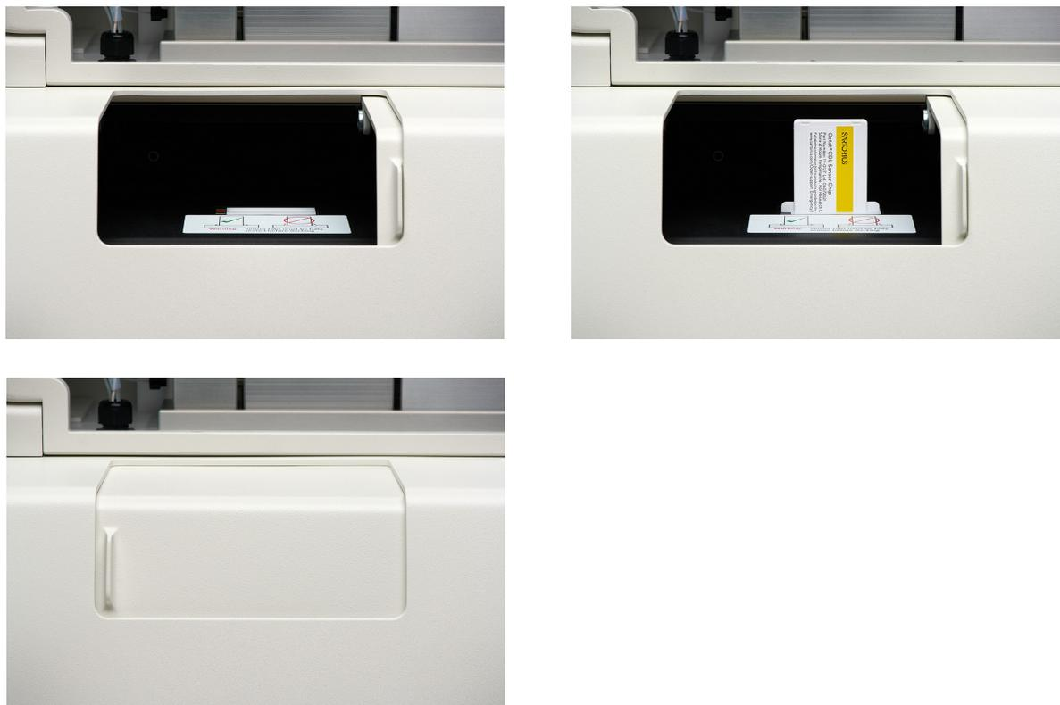
**Figure 4-3:** (Left) Open sensor chip docking door with no sensor chip inserted. (Right) Sensor chip correctly installed with tabs pushed all the way down and the optical sensor light turned off. (Bottom) Closed sensor chip docking door after sensor chip installation.
