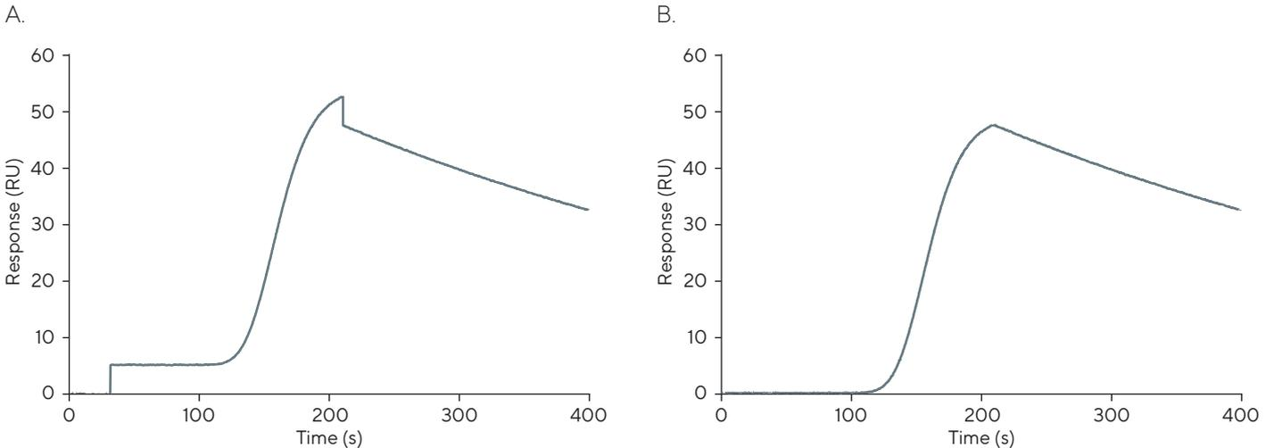
*Note.* (A) Sample OneStep™ sensorgram with a 5 RU RI jump between the sample solution and the running buffer. (B) Buffer exchange of the sample solution into the running buffer can minimize or remove RI jump without the need for double reference subtraction.
