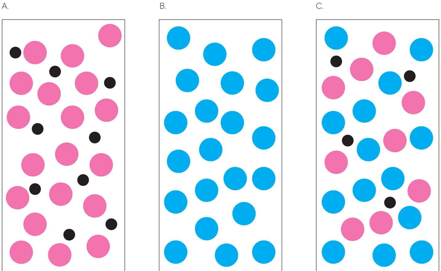
Note. The stock sample solution (A) contains the desired analyte (violet dots) and may also contain excipients or impurities that will be carried over to the sample preparation (black dots). The stock sample solution is mixed into running buffer (B) (blue dots) to create the analyte-containing sample solution at the desired concentration (C).
