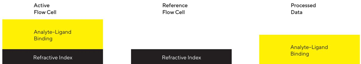
Note. In experiments where the analyte is in a sample buffer that exhibits a low RI, reference subtraction allows the “true” analyte-ligand binding to be assessed.
