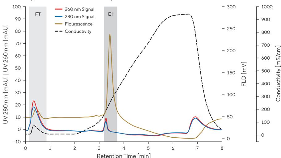
Figure 2: Chromatogram for *Influenza A* Virus Separation on CIMac SO3-0.1 Analytical Column
