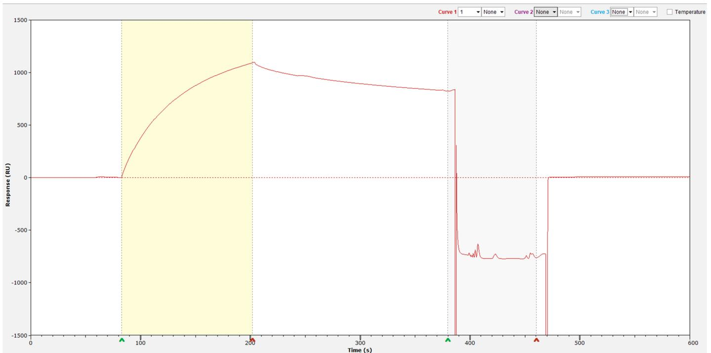
**Figure 7: Sample Recovery Injection Removes Bound Analyte to a User-specified location.** Use of a standard regeneration solution as the recovery solution (20 mM NaOH), flow rate and contact time for Protein A is suitable as a recovery solution for mouse IgG.
