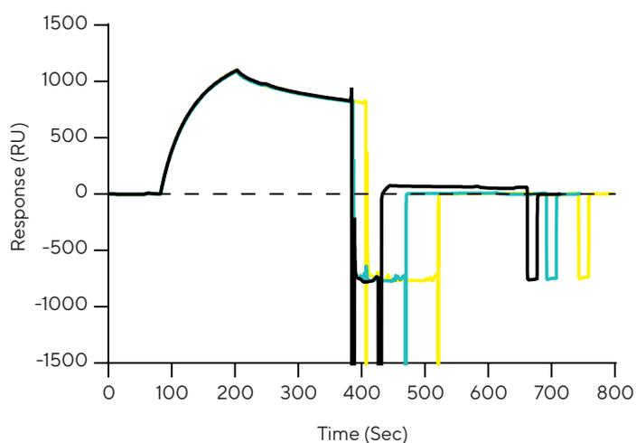
**Figure 8: Increasing the Soak Time Allows more Sample Recovery in the same Volume of Recovery Solution.** Capture of the mouse IgG show excellent reproducibility across injections but as shown, a Sample Recovery Injection with no soak time (black) is not sufficient to remove bound analyte from the surface. Increasing the soak time without changing the flow rate or contact time allows complete recovery of the analyte with a 30 second soak time (teal) or 60 second soak time (yellow).
