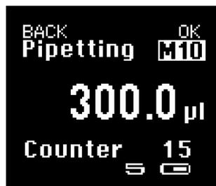
M10 indicates that the pipetting program shown has been saved in memory place 10.
