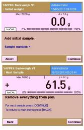
Afterwards, you are prompted to weigh in the first sample. The workflow automatically provides a sample number.
