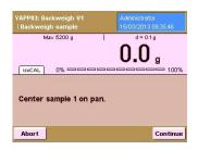
After selecting the sample number, you are prompted to place the corresponding sample on the weighing pan.
