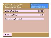
After pressing the menu point 'Initial weighing', you are prompted to place a tare container (e.g. a sample dish, or filter) on the weighing pan. After pressing 'Continue', the container is tared, the value is stored and the display is set to zero.
