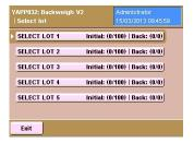
Main menu with the selection of batches. The numbers behind the menu points determine how many samples were already initially weighed or backweighed.
