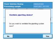
For the Hamilton dispenser YAPP16 stores if a) the instrument has been properly primed to get rid of air bubbles and to fill the syringe and if b) the residual solvent in the syringe is sufficient to perform the next dispensing step. If that's not the case a message screen is shown to user with the question if the sytem should be primed.
