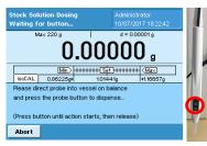
Now the dispenser is ready to apply the solvent to the sample. The user has to direct the probe tip into the sample vial and then to press the probe button.
