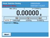
During the filling the application displays the message "Dispenser is filling" to the user. The dispenser stops automatically as soon as the filling process is finished.
