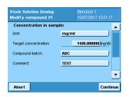
The compound name, molecular weight, purity, unit and target concentration are loaded from the database. The user can modify sample information if required and optionally enter a batch number and a comment for the compound.
