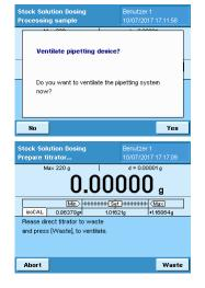
For the Hirschmann opus dispenser YAPP16 stores if a) the instrument has been properly ventilated to get rid of air bubbles and to fill the piston and if b) the residual solvent in the piston is sufficient to perform the next dispensing step. If that's not the case a message screen is shown to user with the question if the sytem should be ventilated.
