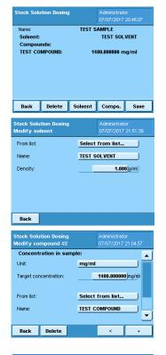
A sample is defined by a combination of at least one compound and a solvent. For the preparation of mixed samples up to 10 compounds can be used. Up to 100 samples can be stored in the YAPP16 database.
