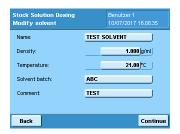
The solvent name and density are loaded from the database. The temperature can be modified by the user. Optionally a batch number and a comment for the solvent can be entered.
