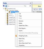
To load weighing results into Chromeleon™ select a sequence file and click the right mouse button. Press "Weighing Scale" in the menu.
