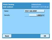
Solvents are defined by name and densits. Up to 100 solvents can be stored in the YAPP16 database.
