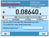
If the administrator has activated the tolerance password approval, the user is forced to enter the password to accept out of tolerance values.
