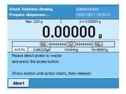
After confirmation with "Yes", the user is asked to direct the probe into a waste vial.
