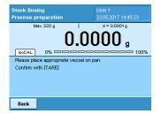
Place a vial on the weighing pan and to tare the balance by pressing hard key <TARE>.
