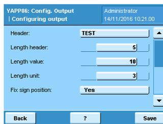
Pressing the "Config" button invokes the configuration menu. The following parameters can be changed in the configuration menu:
