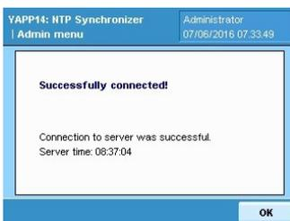
Press the 'Test' button in the configuration menu to check the connection to the NTP server. The time will be not changed at this test, it is just for checking the connection.
