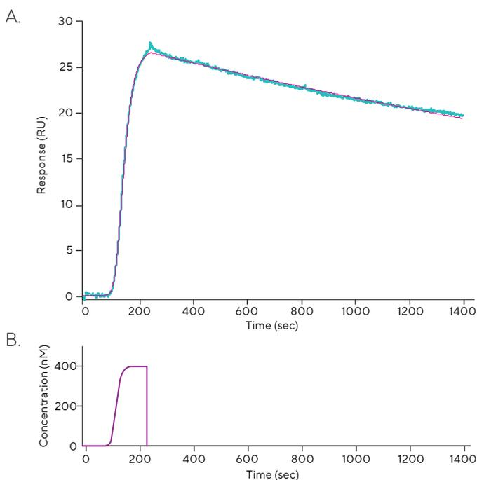
Note. (A) OneStep® Binding data is shown in teal and the 1:1 kinetic model curve is shown in red. (B) The analyte concentration gradient of 0–400 nM is created from a single analyte concentration during a OneStep® Injection.
