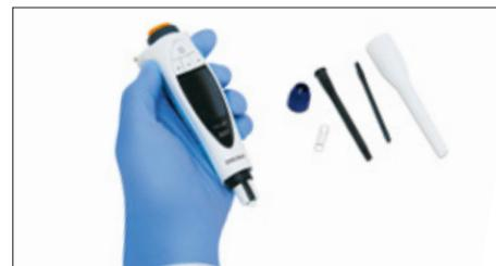
5. After performing the procedure described above, remove the components from the beaker and rinse them with distilled water, then dry preferably in warm air, for at least an hour.
