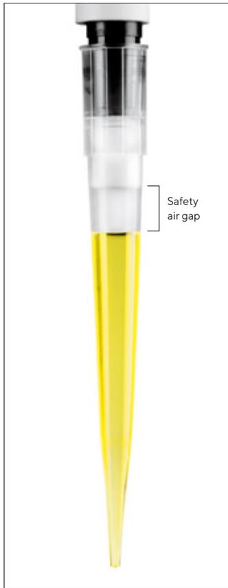
Safetyspace™ Filter Tips offer optimal protection for your work from cross contamination and enable you to use the full volume of the tip with any pipetting mode. They feature the unique Safetyspace™ air gap that leaves additional space between the sample and the filter that conventional filter tips do not have. This extra space prevents the liquid from touching, and permeating, the filter and thus guarantees the pipetting accuracy.
