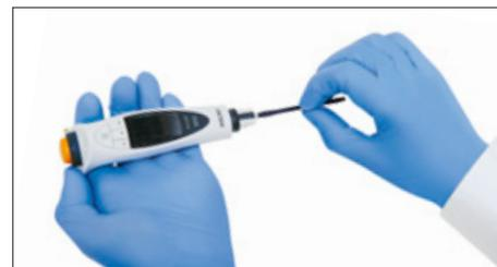
3. Unscrew the piston counter clockwise from the pipette.
