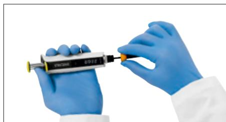
2. Unscrew the tip cone holder counter clockwise and carefully remove it along with the tip cone.
