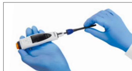
2. Unscrew the tip cone holder counter clockwise and carefully remove the tip cone holder, tip cone and spring.
