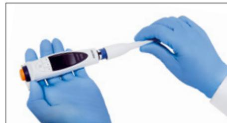
1. Unscrew the tip ejector collar counter clockwise and remove it. Remove the Safe-Cone Filter if fitted.
