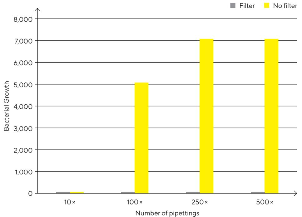
Pipette contamination in pipette interior when pipetting liquid culture of bacteria *Micrococcus Luteus*.
