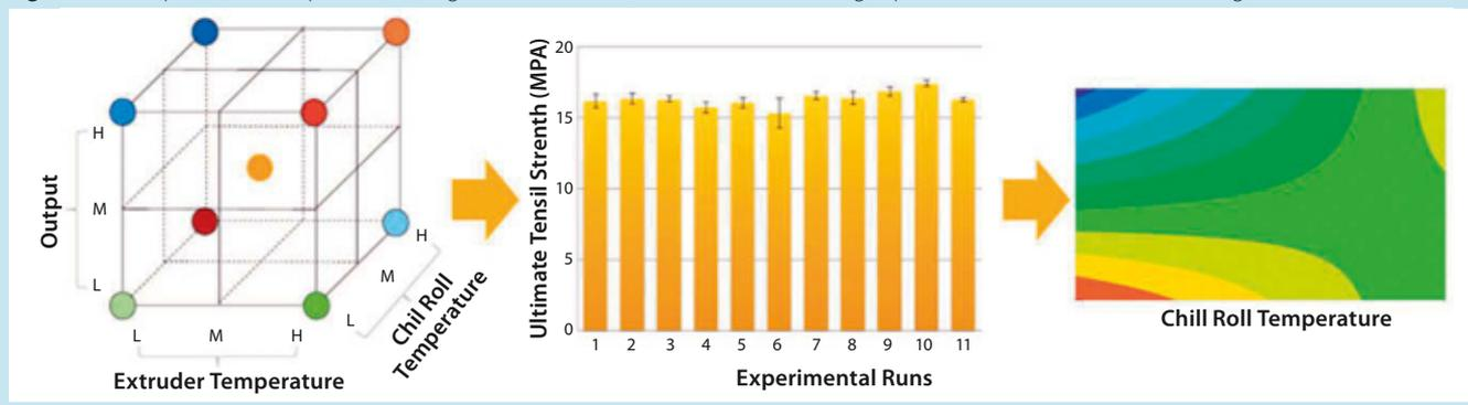
controlled within established ranges. This ensures long-term lot-to-lot consistency for all targeted critical mechanical quality attributes of Flexsafe bags — specifically, strength, flexibility, and (hence) robustness.
