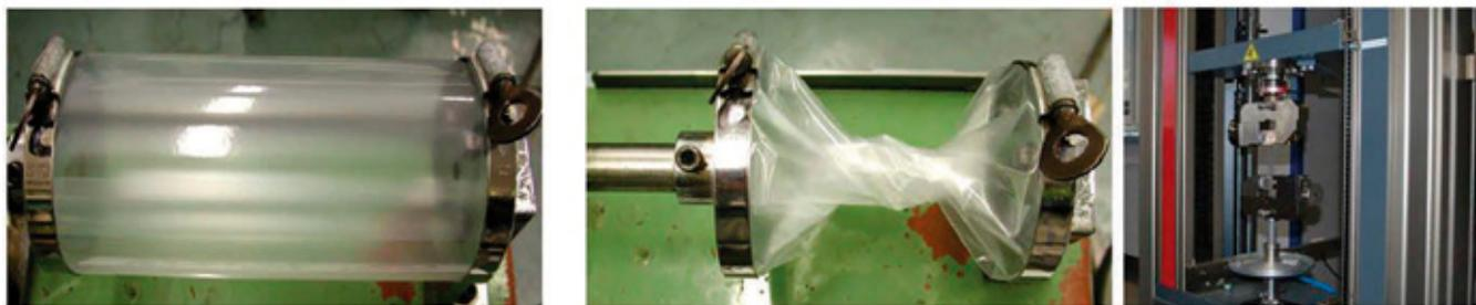
**Photo 2:** Tensile and flex durability tests (photos left and middle from Reference 19)
