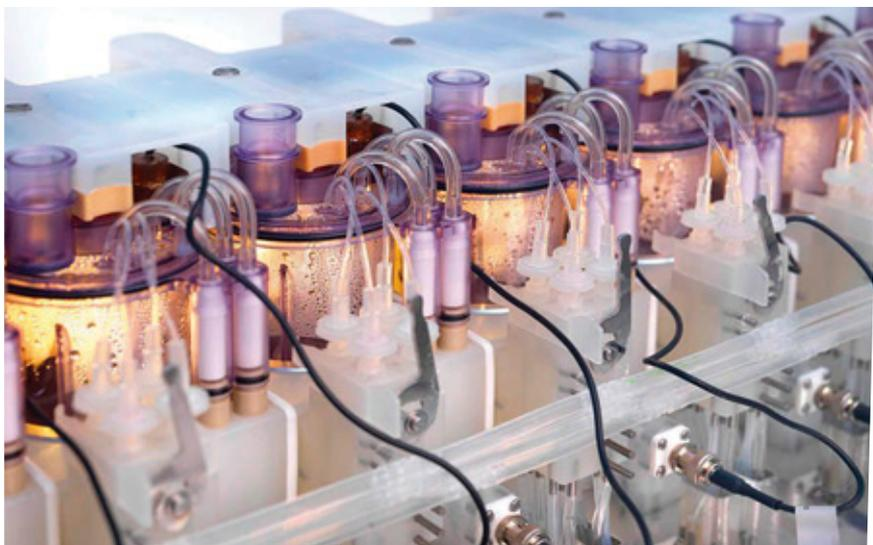
**Photo 2:** The fully automated ambr250 system controls up to 24 × 250-mL bioreactor experiments
