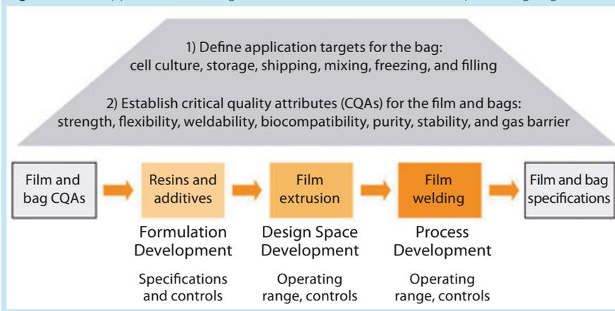
specifications and controls, definition of the film-extrusion process design space, and validation and control of the welding and overall bag-making process.
