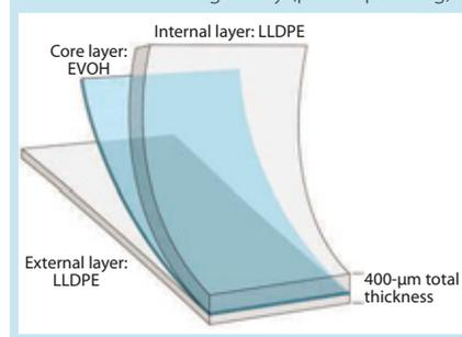
by combining thickness, strength, and flexibility for each layer of S80 film. Together with application knowledge, our resin, film, and bag expertise allowed us to develop a 400- $\mu$ m thick structure that offers outstanding robustness of film, welds, and bags for all bioprocessing applications in upstream production, downstream processing, and final filling.
