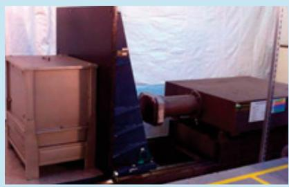
**Figure 9b:** Vehicle vibration ASTM D4728-06, method A (air spectrum)
