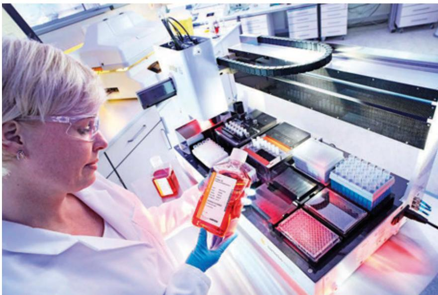
SSB's ambr15 system enables rapid evaluation of 24 or 48 multiple bioreactor cultures at microscale.
