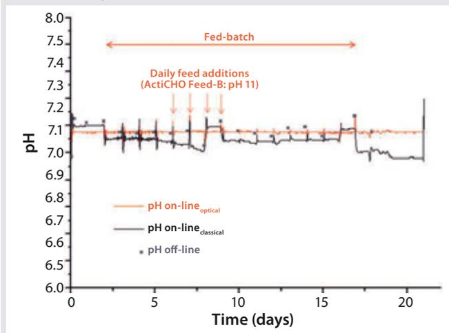
Optical pH sensors have a life time of  $\geq 20,000$  read-outs. At that measuring frequency, continuous measurement over 14 days is possible without any significant loss of performance during cultivation (Figure 7).
