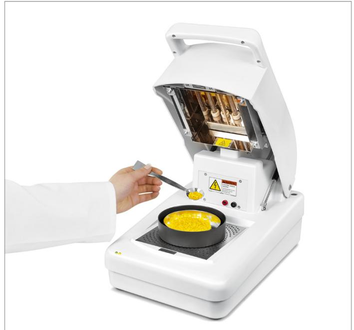
The plastic granules are filled directly into the sample pan without any preparation. A single press of a button starts the measurement process.
