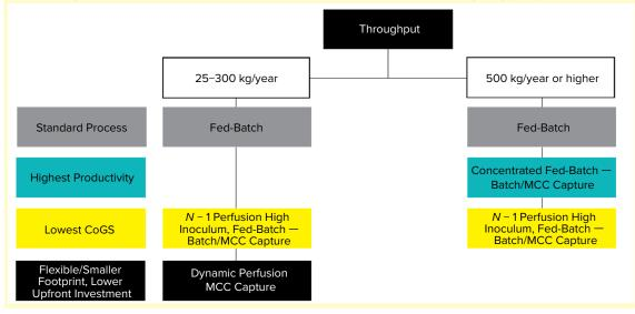
approach to PI, dynamic perfusion offers flexibility for manufacturing multiple molecule types.
