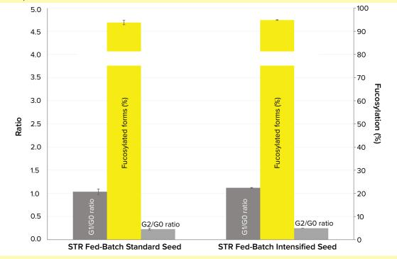
results of the cells cultured in the pilot-scale bioreactor from the intensified seed train show that using HCD cells to seed a pilot-scale bioreactor does not affect product quality. That indicates the usefulness of this approach for a hybrid perfusion/fed-batch process scale-up.
