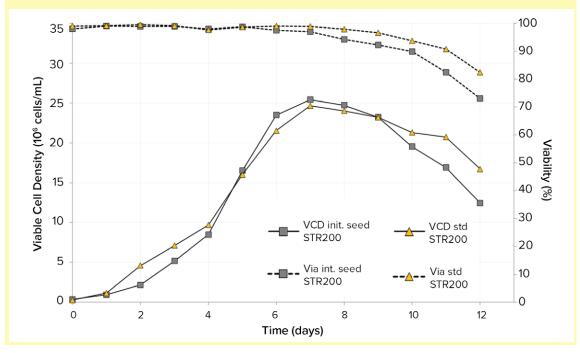
and titer. The results were compared with historical data from a standard seed train for which cells were cultured in standard Biostat RM 20/50 bags (14 L at approximately  $3 \times 10^6$  cells/mL) and used to inoculate a Biostat STR 200 L single-use bioreactor.
