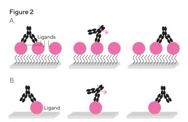
Note. (A) When using a 3D-hydrogel, the potential to crosswalk to another ligand exists if the surface density is too high and will result in an incorrect rate constant being determined during the dissociation phase. (B) Use of a planar sensor chip reduces the surface density and can minimize | remove the avidity effects observed with a 3D-hydrogel sensor chip.
