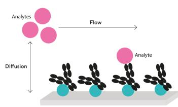
Note. Measurement of binding interactions requires diffusion of the analyte from the bulk flow to the sensor chip surface before binding can be observed.
