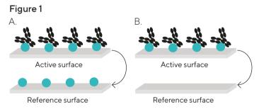
Note. Correct reference surfaces have a large impact on data quality. The capture molecule (teal) should ideally be present on both the active and reference surface to ensure the best data quality possible.
