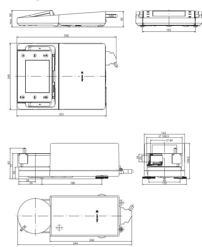
High-capacity Microbalances, Models MSU116P, MSU66S, MSU66P, MSU36S, MSU36P All dimensions are given in millimeters
