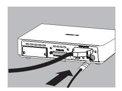
Connecting the Weigh Cell to the Evaluation Unit:Make sure that the connector clicks into place so that the cable is engaged.
