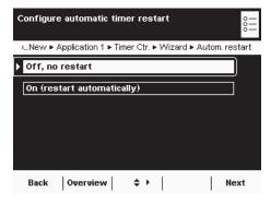
► Specify whether or not there should be an automatic restart after the timer-controlled function has been triggered.
