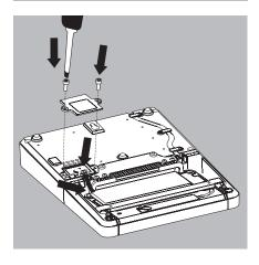
Connect the display and control unit to the electronics module:
