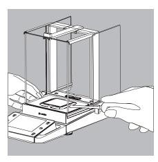
Carefully remove any sample residue/spilled powder using a brush or hand-held vacuum cleaner.
