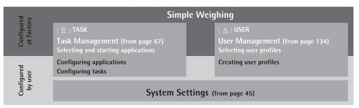
**User Management (USER)** lets you set up user profiles with specific configuration settings and user rights. You can also set up password protection to meet your security requirements. Your balance can also be used without User Management.
