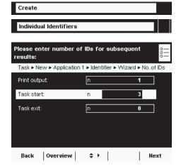
► Enter the desired number of individual IDs that you want to set up. **Print output:** Identifier for the Print 🖪 key
