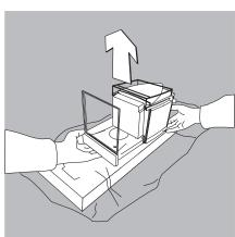
▶ Place one hand under the front panel and the other under the back of the housing and lift the device out of the lower packaging padding.
