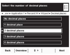
Select accuracy (resolution) for storing value: ▶ New ▶ Application 1 ▶ Percent.W ▶ Wizard ▶ Accuracy Normal resolution 10-fold (+1 dec. place) 100-fold (+2 dec. places)
