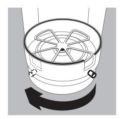
▶ Turn draft shield parts approx. 90 degrees to the left (loosen knurled screw).
