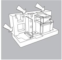
▶ Position the lateral packaging padding around the device and press inward.
