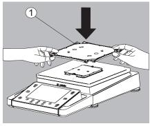
▶ Place the pan support (1) diagonally and press down lightly.
