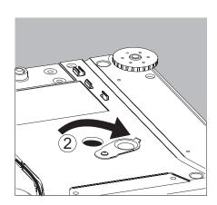
**2.** Push the cover of the below-balance weighing port to one side.
