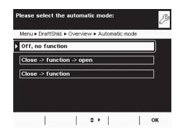
Configure the automatic mode for the draft shield.
