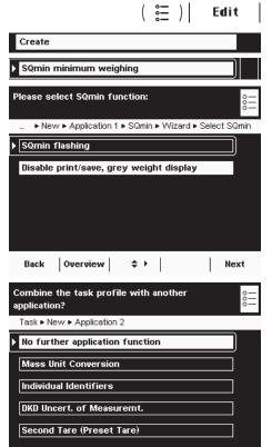
► Select which function should be triggered for minimum sample quantity. **SQmin flashing**: The SQmin tab flashes.
