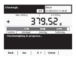
It can be seen immediately on the graphic scale if the result is outside of the tolerance.
