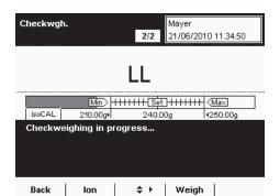
You can toggle between weighing and checkweighing at any time by selecting Weigh or Check.
