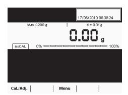
► To open System Settings, select **Menu** when the balance is in operating mode.
