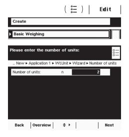
Select the desired number of units (max. 5) to be used to display the weighing results.
