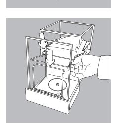
▶ Position the glass panel in the retainers and place it at the back of the draft shield.
