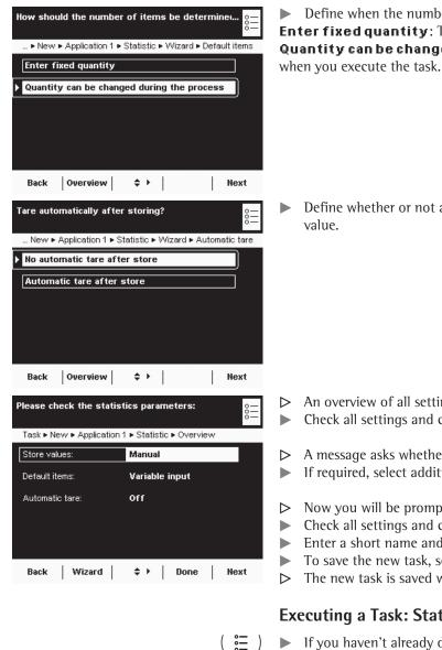
Define when the number of measurements (items) will be set. **Enter fixed quantity:** The item number is defined beforehand. Quantity can be changed during the process: Enter the item number
