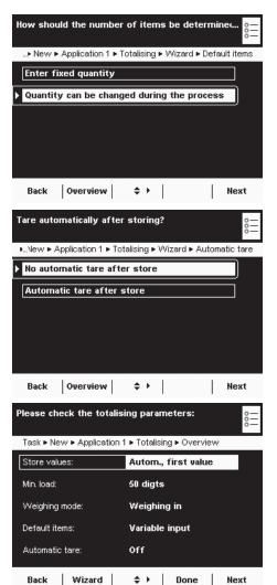
▶ Define when the number of measurements (items) will be set. **Enter fixed quantity:** The quantity of items is defined beforehand. **Quantity can be changed during the process:**
