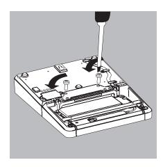
Attach the display and control unit to the electronics module: Reattach the two retaining screws.
