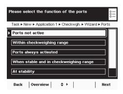
► Define how the ports should be activated depending on the check results \*Ports not active
