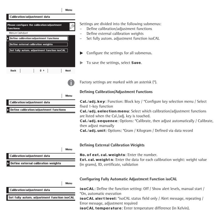
**isoCAL** interval time: Enter interval time in hours.
