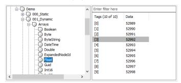
Limitations: only current data is supported for array data. Sartorius has yet to find an OPC UA server that supports historical data for array data. Single dimension arrays are supported (no matrices).
