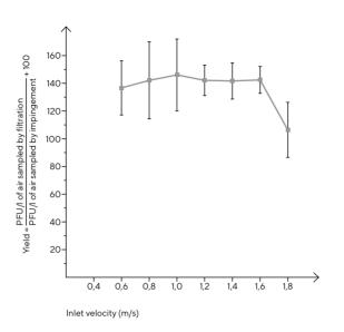
Figure 3 Yield of the gelatin filter after sampling of TI aerosols at 20°C and 55% relative humidity as a function of the inlet velocity at the filter.
