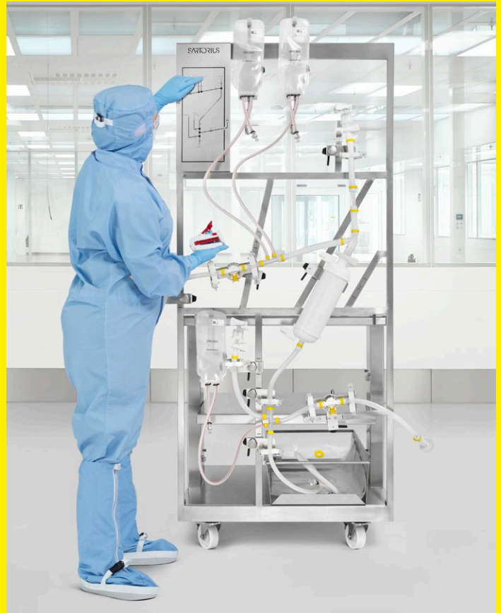
Figure 1: Stainless steel holder with filter transfer set final filling assembly.
