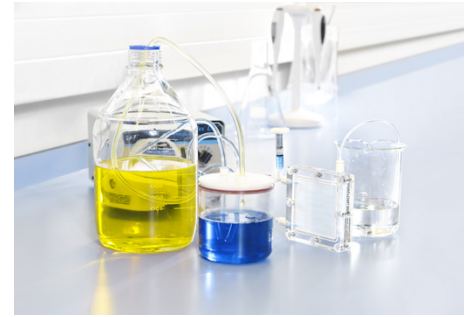
Figure 2: Diafiltration system set up for buffer exchange. Culture medium concentrate can be seen in the center of the image. 1 L 25 mM sodium acetate (exchange buffer) can be seen connected to the system on the left of the image.
