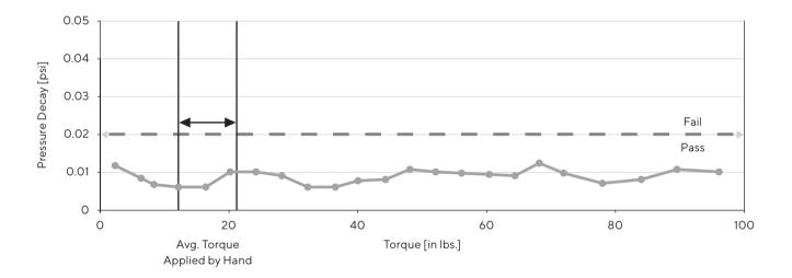
An acceptable leak rate was observed with minimal torque applied, 2 in.-lbs. until material failure at 64 and 100 in-lbs.
