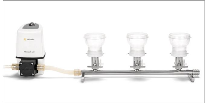
Microsart® Manifold with Microsart® @filter units and Microsart® e.jet Pump
