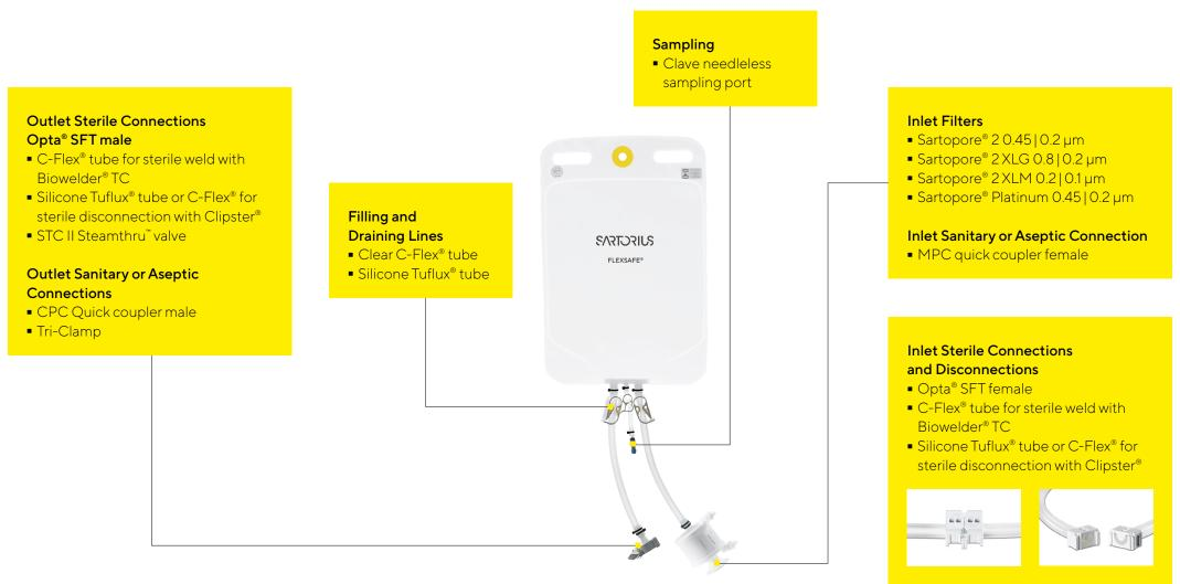
The versatile range of Flexsafe® 2D PDS allows for sterile filtration, storage, shipping and transfer of all biopharmaceutical fluids in all process steps.
