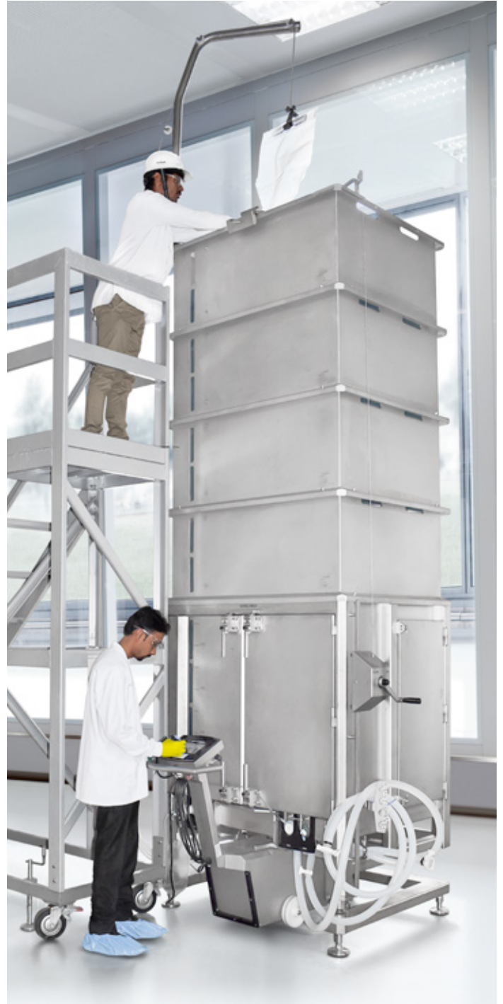
Mixing trial performed at 3000L scale
