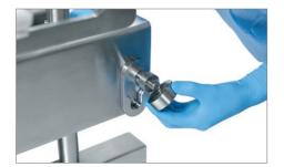
▶ Remove the positioning bars for an easier off-loading of heavy filters.
