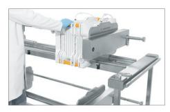
▶ Lift and pull the filters in such a way that the rounded edge on the bottom edge of the filter is supported by the rail that is closest to you.
