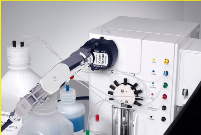
BioPAT ® Spectro flow cell with Kaiser Optical Systems probe connected. Prototype pictured.
