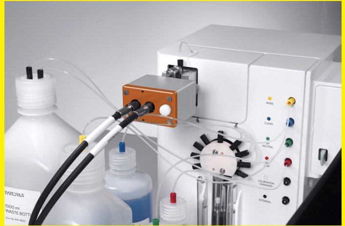
BioPAT ® Spectro flow cell with Tornado Spectral Systems probe connected
