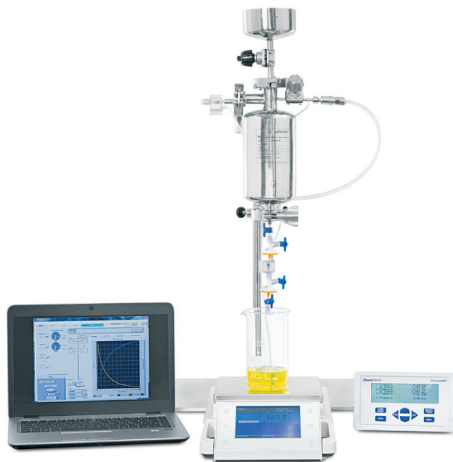
Figure 3: Zero-T set-up for constant pressure filterability trials.
