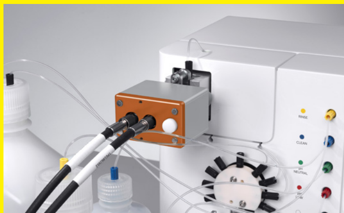
BioPAT® Spectro flow cell with Tornado Spectral Systems probe connected
