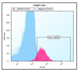
**Step 6: Identify Cells with Depolarized Mitochondrial Membranes.** Mitochondrial depolarization will cause leakage of the dye out of the mitochondria, and the fluorescence intensity of the cell will decrease. Adjust the gate as necessary to encompass the entirely of the left (depolarized) peaks. Depending on the degree of mitochondrial damage, multiple peaks within the "mito damage" gate are possible.
