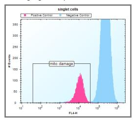
If there are unstained cells on the plate, they may potentially fall inside the "damage" gate due to the low fluorescence intensity of the unstained cells. The size of the gate may need to be decreased to exclude the unstained cells from the "damage" gate.
