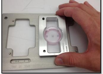
**Tray 25 and holders: A 35 mm dish solution.** This image shows a 35 mm Corning tissue culture dish in the Tray 25 Corning holder. The holder locks the vessel into place to prevent rotation variations when imaging, and to keep the vessel in place during physical marking.
