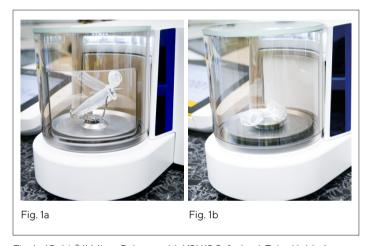
Fig. 1a (Cubis<sup>®</sup> II Micro Balance with YSH13 Safe-Lock Tube Holder) Fig. 1b (Cubis<sup>®</sup> II Micro Balance with standard weighing pan)
