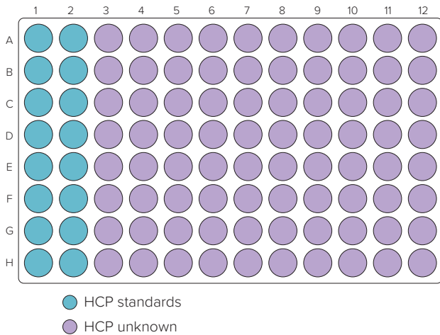
Figure 7: Sample Plate layout for incubation with biosensors on the Sidekick Station.
