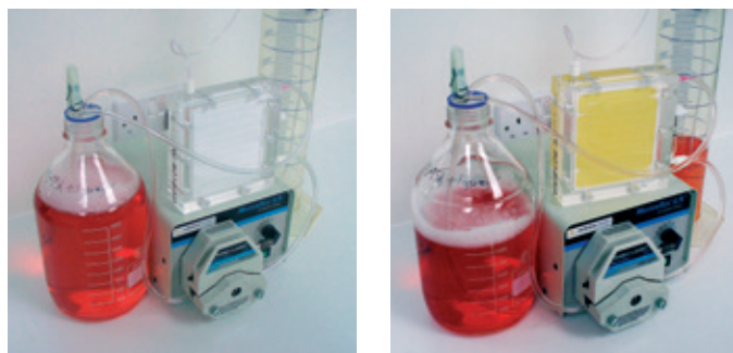
Fig. 1a. and 1 b: Vivaflow ® 200 set up before (1a) and during (1b) the sample concentration process.
