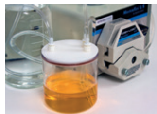
Fig. 2: Diafiltration system set up for buffer exchange. Culture medium concentrate can be seen in the center of the image. 1 L 25 mM Sodium Acetate (exchange buffer) can be seen connected to the system on the left of the image.
