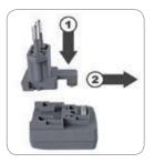
Push (1) and slide (2) to insert the mains adapter required for your power supply into the opening of the AC adapter. When doing this, the mains adapter needs to lock into position.
