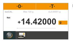
➤ You can read the measured value as soon as the weight value stops changing and the unit is displayed.
