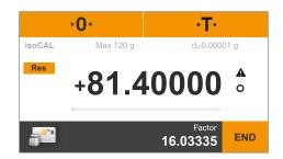
➤ The weight of the sample is multiplied by the entered factor, and the result is displayed.
