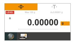
▶ When **LEVEL** appears in red at the top left of the display, you must level the balance.
